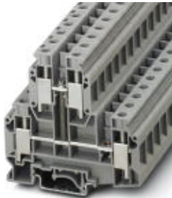
Feed-through terminal block, Cross section: 0.5 mm 2 - 16 mm 2 , AWG: 20 - 6, Connection type: Screw connection, Width: 10.2 mm, Color: gray, Mounting type: NS 35/7,5, NS 35/15, NS 32
