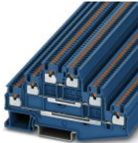
Multi-level terminal block, Cross section: 0.14 mm 2 - 1.5 mm 2 , AWG: 26 - 16, Connection type: Push-in connection, Width: 3.5 mm, Color: blue, Mounting type: NS 35/7,5, NS 35/15
