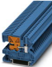
N disconnect terminal block, Screw connection, Cross section: 0.14 mm 2 - 6 mm 2 , AWG: 26 - 10, Width: 6.2 mm, Color: blue, Mounting type: NS 35/7,5, NS 35/15
