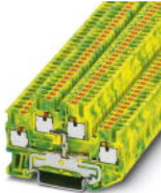
Protective conductor double-level terminal block, Cross section: 0.14 mm 2 - 4 mm 2 , AWG: 26 - 12, Connection type: Push-in connection, Width: 5.2 mm, Color: green-yellow, Mounting type: NS 35/7,5, NS 35/15
