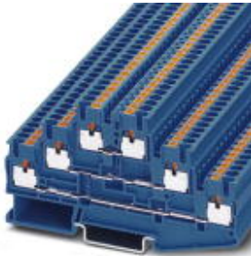
Multi-level terminal block, Connection method: Push-in connection, Cross section: 0.14 mm 2 - 4 mm 2 , AWG: 26 - 12, Width: 5.2 mm, Color: blue, Mounting type: NS 35/7,5, NS 35/15
