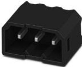
Header, Nominal current: 6 A, Rated voltage (III/2): 160 V, Number of positions: 3, Pitch: 2.5 mm, Color: Black, Contact surface: Tin, Assembly: SMD/THT/THR
