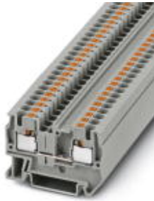
Feed-through terminal block, Connection method: Push-in connection, Cross section: 0.2 mm 2 - 6 mm 2 , AWG: 24 - 10, Width: 6.2 mm, Height: 35.3 mm, Color: gray, Mounting type: NS 35/7,5, NS 35/15
