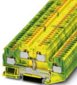
Protective conductor double-level terminal block, Cross section: 0.2 mm 2 - 6 mm 2 , AWG: 24 - 10, Connection type: Push-in connection, Width: 6.2 mm, Color: green-yellow, Mounting type: NS 35/7,5, NS 35/15
