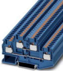
Double-level terminal block, Cross section: 0.2 mm 2 - 6 mm 2 , AWG: 24 - 10, Connection type: Push-in connection, Width: 6.2 mm, Color: blue, Mounting type: NS 35/7,5, NS 35/15
