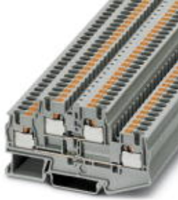
Double-level terminal block, Cross section: 0.2 mm 2 - 6 mm 2 , AWG: 24 - 10, Connection type: Push-in connection, Width: 6.2 mm, Color: gray, Mounting type: NS 35/7,5, NS 35/15
