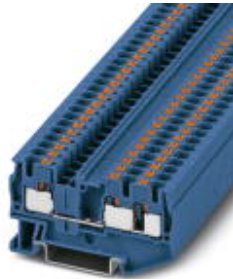
Feed-through terminal block, Connection method: Push-in connection, Cross section: 0.2 mm 2 - 6 mm 2 , AWG: 24 - 10, Width: 6.2 mm, Color: blue, Mounting type: NS 35/7,5, NS 35/15
