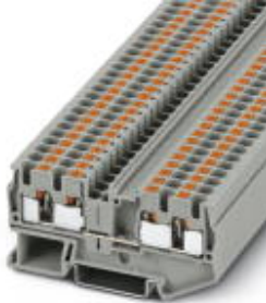
Feed-through terminal block, Connection method: Push-in connection, Cross section: 0.2 mm 2 - 6 mm 2 , AWG: 24 - 10, Width: 6.2 mm, Height: 35.3 mm, Color: gray, Mounting type: NS 35/7,5, NS 35/15
