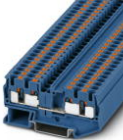
Feed-through terminal block, Connection method: Push-in connection, Cross section: 0.2 mm 2 - 6 mm 2 , AWG: 24 - 10, Width: 6.2 mm, Height: 35.3 mm, Color: blue, Mounting type: NS 35/7,5, NS 35/15
