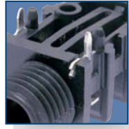
Chassis ground contact
