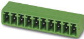
Header, Nominal current: 8 A, Rated voltage (III/2): 160 V, Number of positions: 2, Pitch: 3.81 mm, Color: green, Contact surface: Tin, Assembly: Soldering
