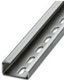
G-profile DIN rail, material: Steel, perforated, height 15 mm, width 32 mm, length 2 m
