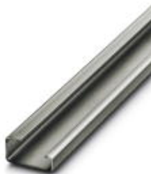
G-profile DIN rail, material: Steel, unperforated, height 15 mm, width 32 mm, length 2 m
