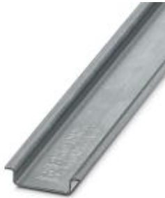
DIN rail, material: Galvanized, unperforated, height 7.5 mm, width 35 mm, length: 2 m
