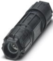
QUICKON cable connector, black, 3-pos. +PE, 1.0 mm 2 ... 2.5 mm 2 / 630 V / 20 A, for cable diameters of 6 mm ... 10 mm.
