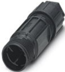
QUICKON cable connector, black, 3-pos. +PE, 1.0 mm 2 ... 2.5 mm 2 / 630 V / 20 A, for cable diameters of 9 mm ... 14 mm.
