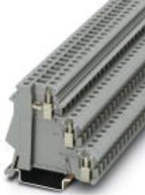
Sensor/actuator terminal block, Cross section: 0.2 mm 2 - 4 mm 2 , AWG: 24 - 12, Connection type: Screw connection, Width: 6.2 mm, Color: gray, Mounting type: NS 35/7,5, NS 35/15
