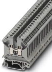
Feed-through terminal block, Connection method: Screw connection, Cross section: 0.2 mm 2 - 6 mm 2 , AWG: 24 - 10, Width: 6.2 mm, Color: gray, Mounting type: NS 35/7,5, NS 35/15, NS 32
