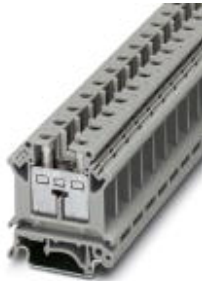
Feed-through terminal block, Screw connection, Cross section: 2.5 mm 2 - 25 mm 2 , AWG: 12 - 4, Width: 12.2 mm, Color: gray, Mounting type: NS 35/7,5, NS 35/15, NS 32
