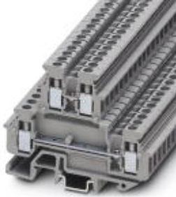
Feed-through terminal block, Cross section: 0.2 mm 2 - 4 mm 2 , AWG: 24 - 12, Connection type: Screw connection, Width: 5.2 mm, Color: gray, Mounting type: NS 15
