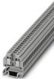
Feed-through terminal block, Connection method: Screw connection, Cross section: 0.14 mm 2 - 1.5 mm 2 , AWG: 26 - 16, Width: 4.2 mm, Color: gray, Mounting type: NS 15
