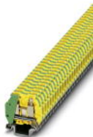
Ground modular terminal block, Connection method: Screw connection, Cross section: 0.14 mm 2 - 1.5 mm 2 , AWG: 26 - 16, Width: 4.2 mm, Color: green-yellow, Mounting type: NS 15
