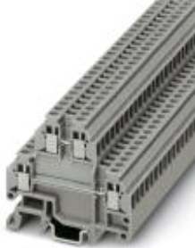
Feed-through terminal block, Cross section: 0.14 mm 2 - 1.5 mm 2 , AWG: 26 - 16, Connection type: Screw connection, Width: 4.2 mm, Color: gray, Mounting type: NS 15, NS 35/7,5, NS 35/15
