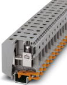
Feed-through terminal block, Connection method: Screw connection, Cross section: 16 mm 2 - 70 mm 2 , AWG: 6 - 2/0, Width: 20 mm, Height: 75.8 mm, Color: gray, Mounting type: NS 35/15, NS 32
