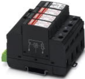
Surge voltage arrester consisting of base element with remote indicator contact and ground connectors, for mounting on NS 35/7.5, nominal voltage: 230 V AC, 3 + 1 circuit
