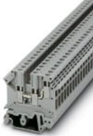
1-level terminal block with double connection on one side, cross section: 0.2 - 4 mm 2 , AWG: 24 - 12, width: 6.2 mm, color: gray
