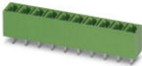
Header, Nominal current: 8 A, Rated voltage (III/2): 320 V, Number of positions: 12, Pitch: 5.08 mm, Color: green, Contact surface: Tin, Assembly: Soldering
