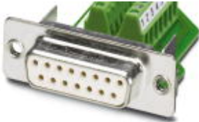
D-SUB contact insert, shell size 2, with 15 signal contacts, female contact type, screw connection, straight, for panel mounting frame and sleeve housing with IP67 protection
