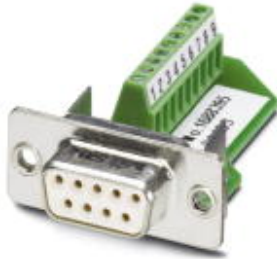
D-SUB contact insert, shell size 1, with 9 signal contacts, female contact type, screw connection, straight, for panel mounting frame and sleeve housing with IP67 protection
