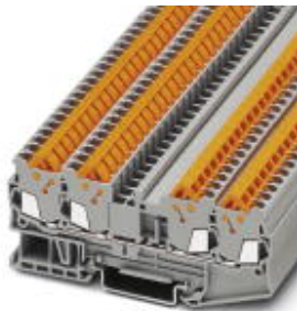
Feed-through terminal block, Connection method: Quick connection, Cross section: 0.25 mm 2 - 1.5 mm 2 , AWG: 24 - 16, Width: 5.2 mm, Color: gray, Mounting type: NS 35/7,5, NS 35/7,5
