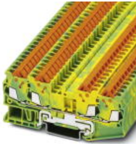
Ground modular terminal block, Connection method: Quick connection, Cross section: 0.25 mm 2 - 1.5 mm 2 , AWG: 24 - 16, Width: 5.2 mm, Color: green-yellow, Mounting type: NS 35/7,5, NS 35/7,5
