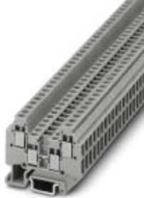
Feed-through terminal block, Cross section: 0.14 mm 2 - 1.5 mm 2 , AWG: 26 - 16, Connection type: Screw connection, Width: 4.2 mm, Color: gray, Mounting type: NS 15
