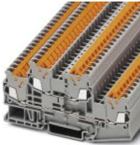
Feed-through terminal block, Cross section: 0.25 mm 2 - 1.5 mm 2 , AWG: 24 - 16, Connection type: Quick connection, Width: 5.2 mm, Color: gray, Mounting type: NS 35/7,5, NS 35/15
