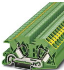
Installation level terminal block, Spring-cage connection, Cross section: 0.2 mm 2 - 16 mm 2 , AWG: 24 - 6, Width: 10 mm, Color: green-yellow, Mounting type: NS 35/7,5, NS 35/15
