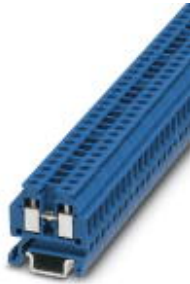
Feed-through terminal block, Connection method: Screw connection, Cross section: 0.14 mm 2 - 1.5 mm 2 , AWG: 26 - 16, Width: 4.2 mm, Color: blue, Mounting type: NS 15
