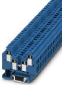
Feed-through terminal block, Cross section: 0.14 mm 2 - 1.5 mm 2 , AWG: 26 - 16, Connection type: Screw connection, Width: 4.2 mm, Color: blue, Mounting type: NS 15
