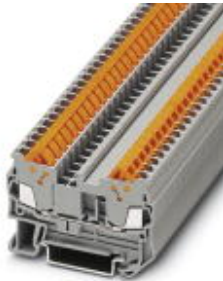
Fast connection terminal block, Connection method: Quick connection, Cross section: 0.25 mm 2 - 1.5 mm 2 , AWG: 24 - 16, Width: 5.2 mm, Color: gray, Mounting type: NS 35/7,5, NS 35/15
