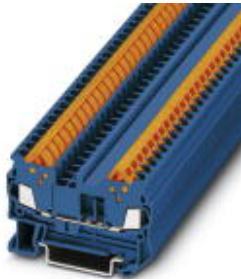
Feed-through terminal block, Connection method: Quick connection, Cross section: 0.25 mm 2 - 1.5 mm 2 , AWG: 24 - 16, Width: 5.2 mm, Color: blue, Mounting type: NS 35/7,5, NS 35/15
