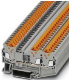
Feed-through terminal block, Connection method: Quick connection, Cross section: 0.25 mm 2 - 1.5 mm 2 , AWG: 24 - 16, Width: 5.2 mm, Color: gray, Mounting type: NS 35/7,5, NS 35/7,5
