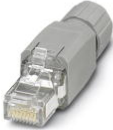
RJ45 connector, IP20, CAT5e, 8-pos., with QUICKON fast connection technology, for 26 ... 23 AWG 1-wire and 7-wire conductors, for 4.5 mm ... 8.0 mm cable diameter, labeling: TIA 568 B, color: gray
