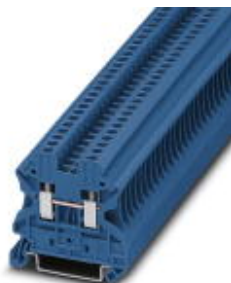
Feed-through terminal block, Connection method: Screw connection, Cross section: 0.14 mm 2 - 4 mm 2 , AWG: 26 - 12, Width: 5.2 mm, Color: blue, Mounting type: NS 35/7,5, NS 35/15
