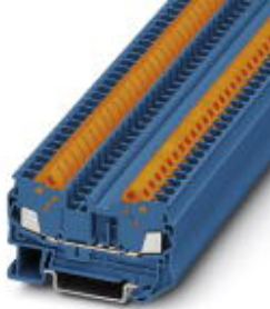
Feed-through terminal block, Connection method: Quick connection, Cross section: 0.5 mm 2 - 2.5 mm 2 , AWG: 20 - 14, Width: 6.2 mm, Color: blue, Mounting type: NS 35/7,5, NS 35/15
