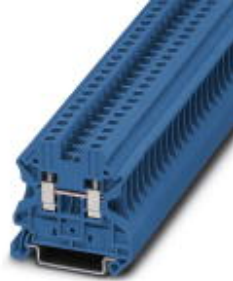
Feed-through terminal block, Connection method: Screw connection, Cross section: 0.14 mm 2 - 6 mm 2 , AWG: 26 - 10, Width: 6.2 mm, Color: blue, Mounting type: NS 35/7,5, NS 35/15
