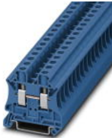
Feed-through terminal block, Connection method: Screw connection, Cross section: 0.2 mm 2 - 10 mm 2 , AWG: 24 - 8, Width: 8.2 mm, Color: blue, Mounting type: NS 35/7,5, NS 35/15
