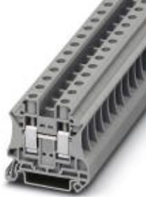
Feed-through terminal block, Connection method: Screw connection, Cross section: 0.5 mm 2 - 16 mm 2 , AWG: 20 - 6, Width: 10.2 mm, Height: 46.9 mm, Color: gray, Mounting type: NS 35/7,5, NS 35/15
