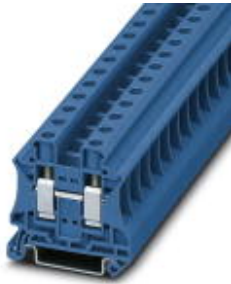
Feed-through terminal block, Connection method: Screw connection, Cross section: 0.5 mm 2 - 16 mm 2 , AWG: 20 - 6, Width: 10.2 mm, Height: 46.9 mm, Color: blue, Mounting type: NS 35/7,5, NS 35/15
